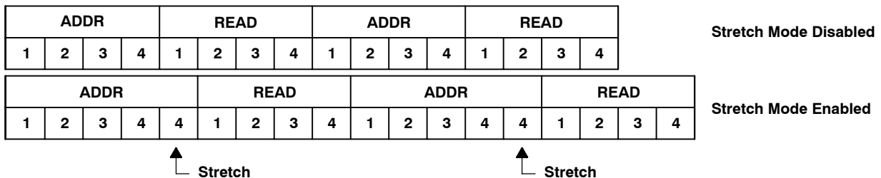
Figure 5. Two 32-Bit Nonpage-Mode Reads
