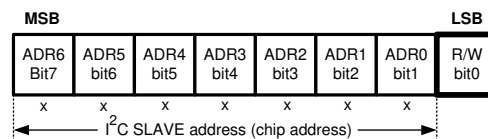
Figure 6-42. Address and Read/Write Bit
