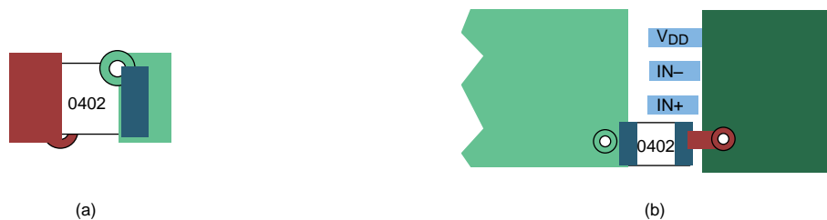
Figure 21. Typical Decoupling Capacitor Layouts
