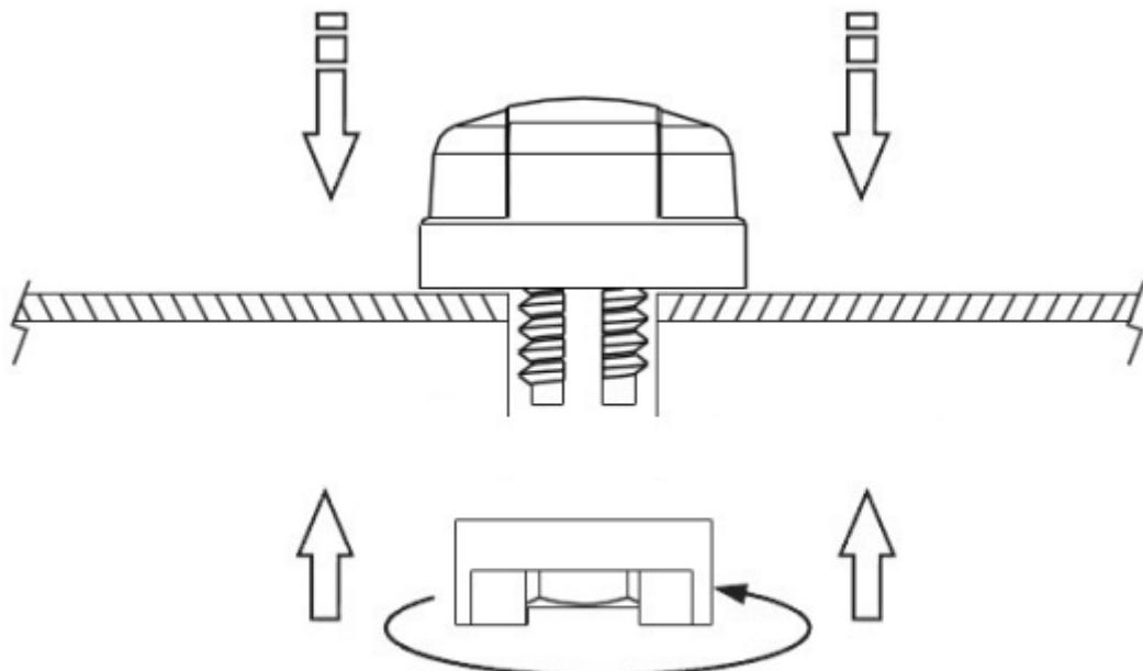
Recommended torque for Mounting is 24.5N·m
