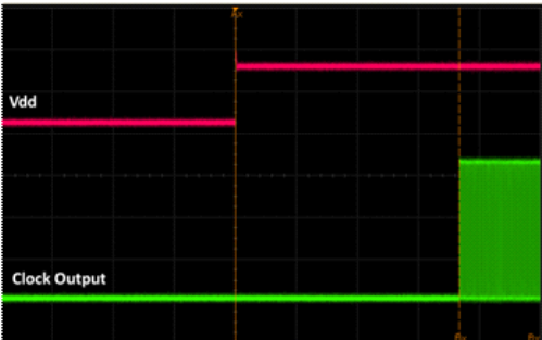
Figure 16. Startup Waveform vs. Vdd
