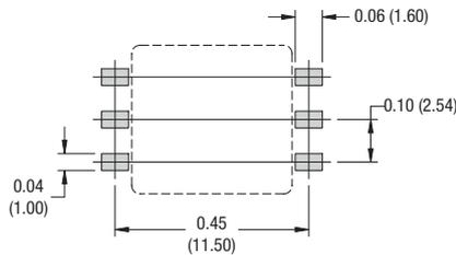
Unless otherwise stated all dimensions in inches (mm)  $\pm 0.01$  (0.25). All pins on a 0.1 (2.54) pitch and within  $\pm 0.01$  (0.25) of true position.
