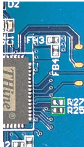
Figure 8 THCV242A-P I2C Target Address Setting Resistors
