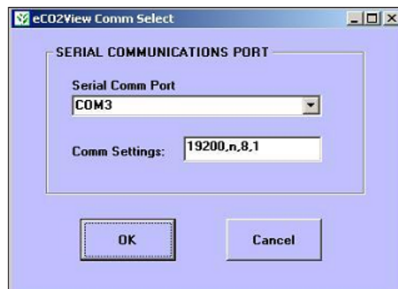
Figure 19: Serial Communications Port Window
