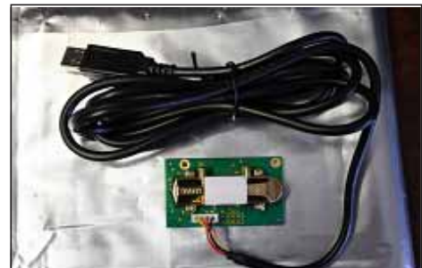
Figure 6: T6613/6615 CO 2 Sensor Connected to USB Cable
