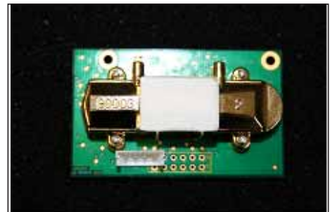
Figure 5: T6613/6615 CO 2 Sensor with 4 Pin Header
