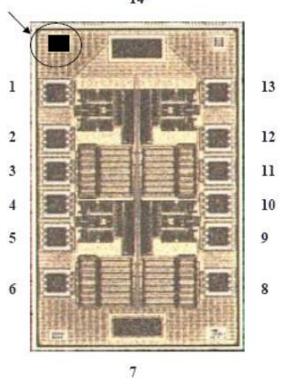
Pad size: Pad numbers 1 to 6 and 8 to 13:  $100 \times 100 \ \mu m$ Pad numbers 7 (GND) and 14 (Vcc):  $100 \times 280 \mu m$
