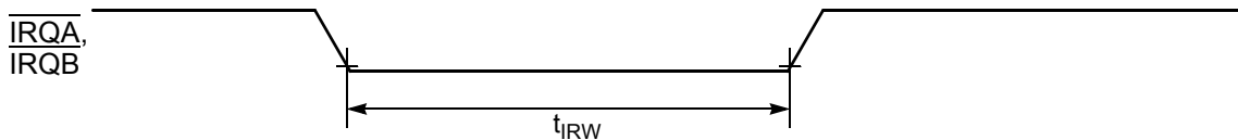
Figure 10-6 External Interrupt Timing (Negative-Edge Sensitive)
