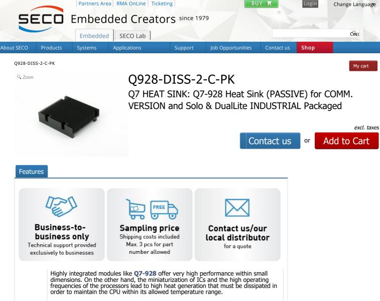
The operating temperature specified in the Technical Features of Q7-928 indicates the temperature range in which any and all parts of the heat spreader / heat sink must remain, in order for SECO to guarantee functionality. Hence, these numbers do not necessarily indicate the suitable environmental temperature.
