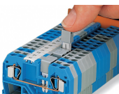
Commoning using an adjacent jumper. Push jumper down until fully inserted!
