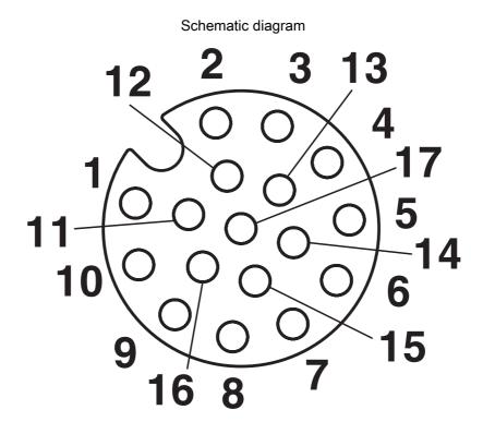
Pin assignment M12, 17-pos., socket side view
