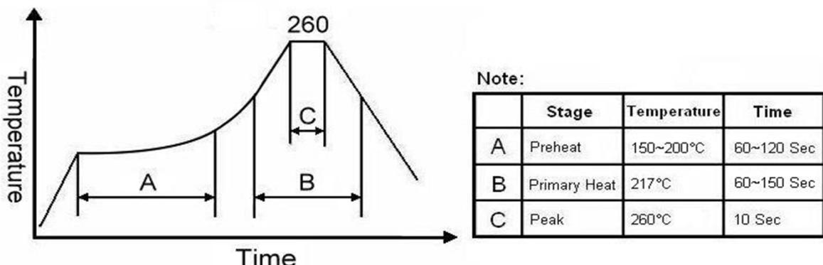
For soldering reflow profile and reliability test ratings go to: <http://www.pericom.com/pdf/sre/reflow.pdf>
