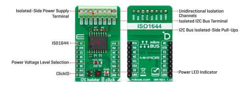
ISO1644 supports I2C 2-Wire bidirectional data transfer between a host device and several peripheral devices, where the host MCU controls the bus, specifically the serial clock (SCL) line. The data transfer can be made in standard, fast, fast-mode plus, and high-speed mode with speeds up to 3.4Mbps. As for three GPIO lines, the ISO1644 consists of two lines in one direction and one in the opposite direction. It could be used for any GPIO purpose.
