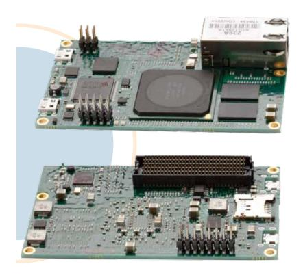
The EP1011xS board create is a compact, cost-effective, and powerful platform for developing high performance networked control platforms. At only 3.5" x 2.2" x 1.0", the board will fit into compact spaces, while 1 serial port, 2 USB ports, and 1 Gigabit Ethernet port plus the EBC connector provide the necessary control I/O.
