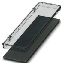
DIN rail housing for use in distribution boards in accordance with DIN 43880, transparent hinged cover, can be sealed, including insertion plate, width: 161.6 mm, height: 45 mm, depth: 8 mm, color: black (similar RAL 9005)
