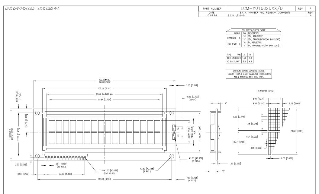
\*UNLESS OTHERWISE SPECIFIED TOLERANCES PER DECIMAL PRECISION ARE: X=±1 (±0.039), X.X=±0.5 (±0.020), X.XX=±0.25 (±0.010), X.XXX=±0.127 (±0.005). LEAD SIZE=±0.05 (±0.002), LEAD LENGTH=±0.75 (±0.030). MIN= +DECIMAL PRECISION MAX.= ±0.000 + DECIMAL PRECISION MAX.= ±0.
