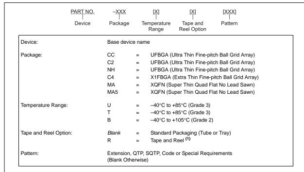
Note 1: Tape and Reel identifier only appears in the catalog part number description. This identifier is used for ordering purposes and is not printed on the device package. See "Orderable Part Numbers" below or check with your Microchip Sales Office for package availability with the Tape and Reel option.
