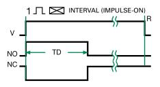
NC = Normally Closed Contact t = IncompleteTime Delay TD,TD1,TD2 =Time Delay **C** = Count **P** = Pulse Duration  $-\langle \rangle = Undefined Time$
