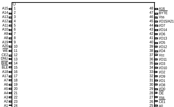
Figure 1. 48-pin TSOP I pinout (Front View) [1, 2]
