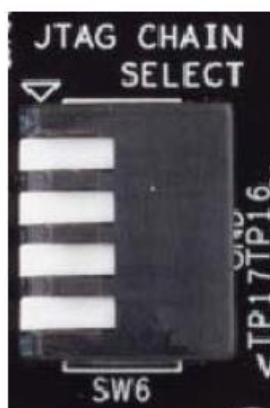
Figure 5.1. PCI Express Board Configuration/Programming Mux Selection
