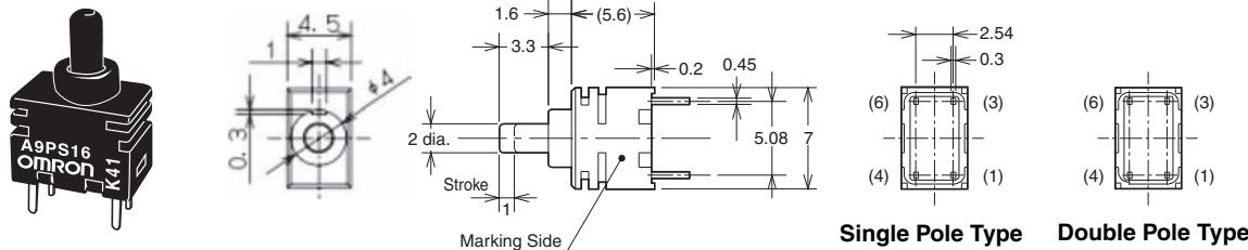
Note: NO.(4) and (6) terminals in the SPDT models are dummies to support the Switch case.
