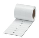
Label for rough surfaces, Roll, white, unlabeled, can be labeled with: THERMOMARK E.300 (D)/600 (D), THERMOMARK ROLL 2.0, THERMOMARK ROLL, THERMOMARK ROLL X1, THERMOMARK ROLLMASTER 300/600, THERMOMARK X1.2, mounting type: adhesive, Number of individual labels: 2500, text field height: 12 mm, text field width: 26.5 mm
