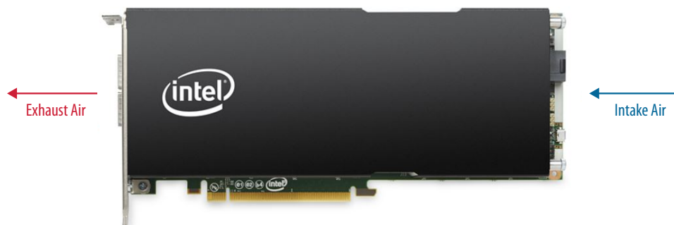
Figure 7. Intel FPGA PAC D5005 Airflow Pattern
