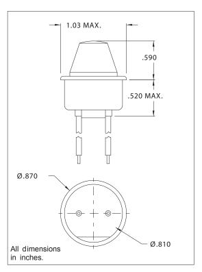
Mounting: Supplied with speednut SN2089. Mounting hole pattern on page SP2.
