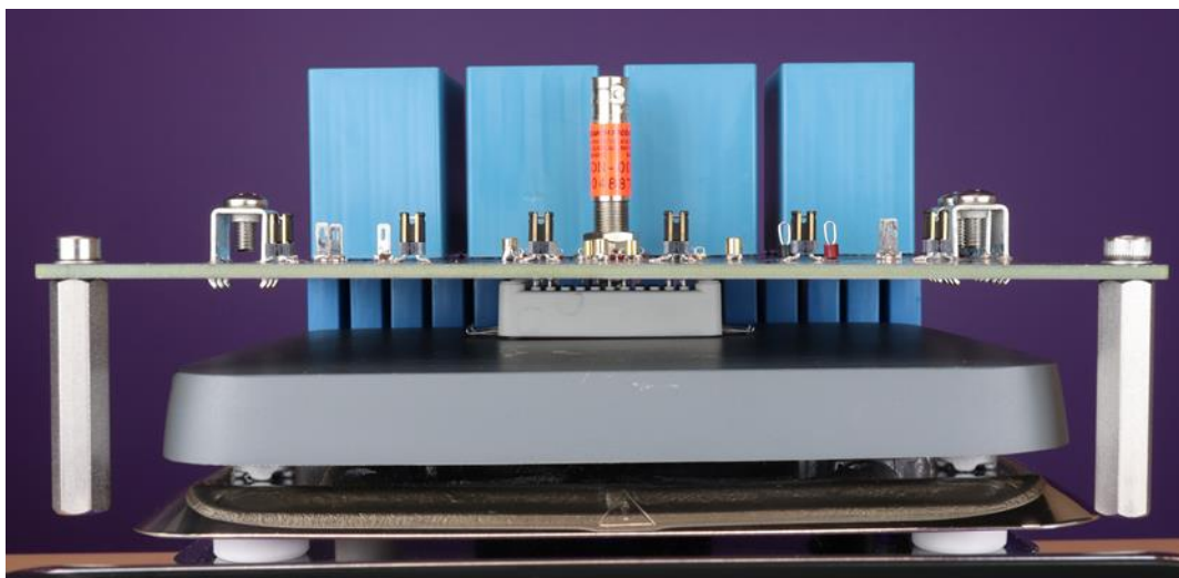
FIGURE 13: FM3 MODULE ON HOT PLATE FOR ELEVATED TEMPERATURE TESTING
