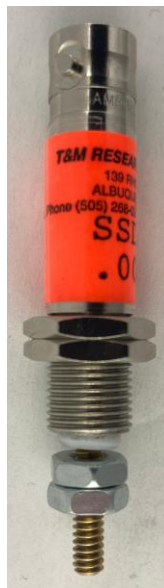
FIGURE 5: T&M RESEARCH SSDN-005 5 m \Omega CVR
