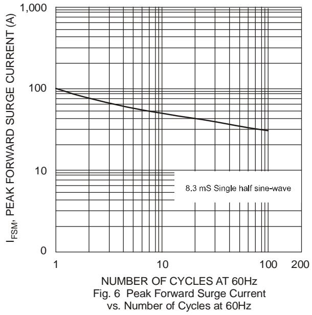
Fig. 6 Peak Forward Surge Current vs. Number of Cycles at 60Hz
