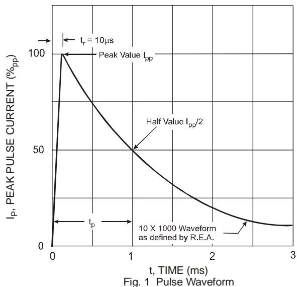
Fig. 1 Pulse Waveform
