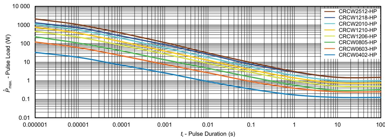
Maximum pulse load, continuous pulses; applicable if  $\bar{P} \leq P(\vartheta_{\text{amb}})$  and  $\hat{U} \leq \hat{U}_{\max.}$ ;
