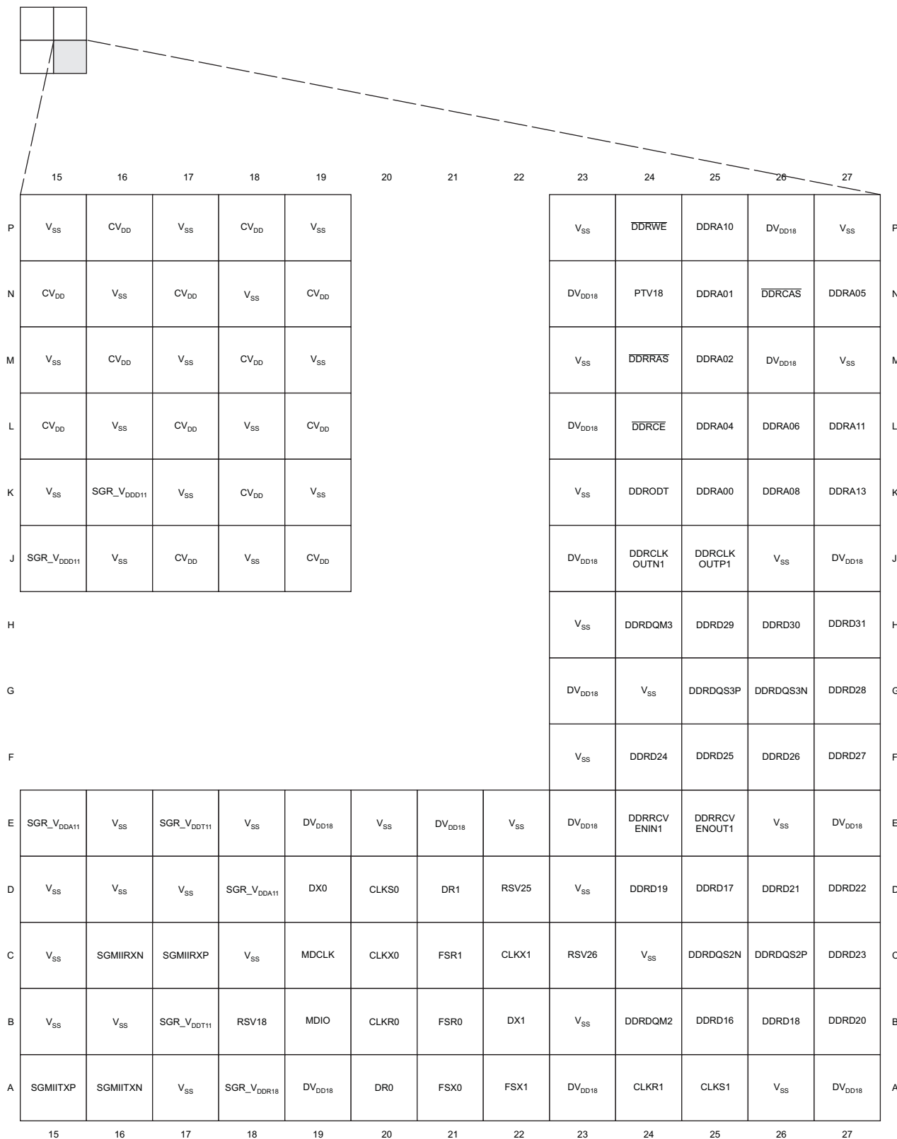
Figure 2-4. TCI6487/8 Pin Map (Bottom View) [Quadrant C]
