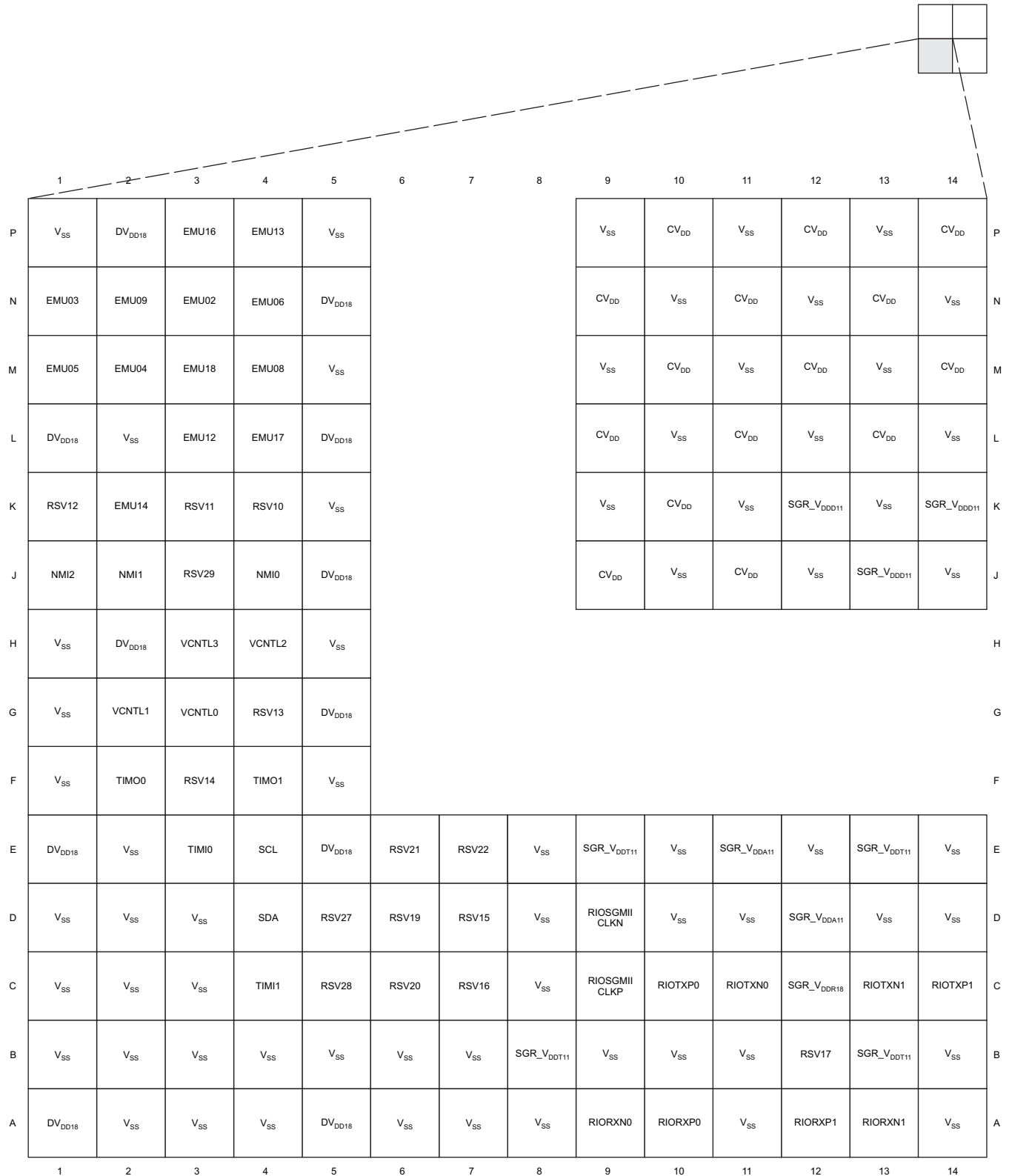
Figure 2-5. TCI6487/8 Pin Map (Bottom View) [Quadrant D]
