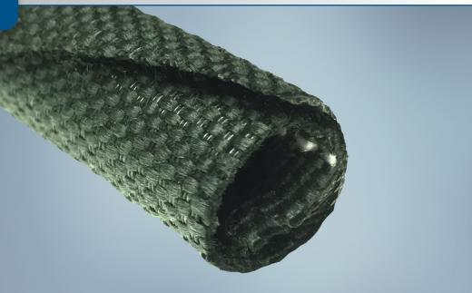
**ROUNDIT® 2000 NX** is a woven combination of Nomex® and PPS (polyphenylene sulfide). The Nomex®/PPS blend in a flat weave construction gives ROUNDIT 2000 NX a rugged yet smooth texture and appearance for high temperature bundling and abrasion resistance. This product is rated to +200°C (+392°F) and is non-halogenated.
