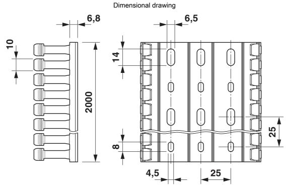
Base perforation according to DIN EN 50085
