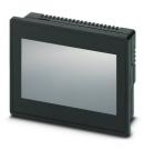
Web panel with 10.92 cm / 4.3" TFT-display (analog resistive), 480 x 272 pixel(s) (WQVGA), 16. 7 million colors, i.MX 6DualLite, 1 GHz, 1x USB Host 2.0, 1 x Ethernet (10/100 Mbps), RJ45, Yocto/Linux and user software: QT browser. (bus system: without)
