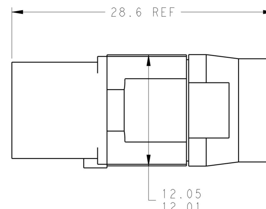
1) FRONT & REAR INSULATORS: HIGH-TEMP THERMOPLASTIC OR THERMOSET EPOXY PER ASTM D5948. CONTACT RETENTION CLIPS: STAINLESS STEEL PER AISI 302 OR COPPER ALLOY PER ASTM B194, REAR GROMMET: FLUOROSILICONE ELASTOMER PER MIL-R-25988 B EXCEPT 4.6.6.1.
