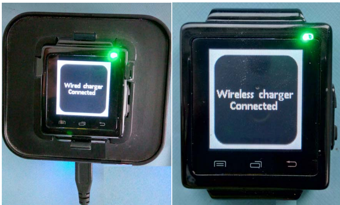
Figure 3: Wired and Wireless Charging Indication
