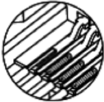
Insufficient amount of solder used
