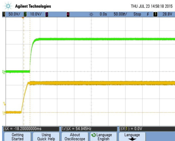
Turn-on transient at zero load current (50 mS/div, Top Trace: Vout, 10V/div; Bottom Trace: Vin, 50V/div)
