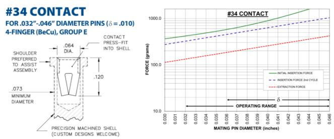
The insertion / extraction force characteristics above were derived using a 30 microinch gold-plated contact and polished steel gauge pins having a bullet-shaped tip. The curves represent typical average values; they are best used to compare the differences between similar size contacts and to guide you in selecting one that is suitable for your application. Your results may vary, so for your specification, we encourage you to obtain complimentary samples for your evaluation.
