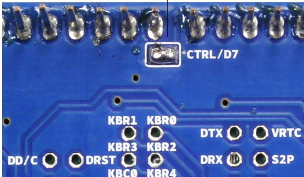
Bridged pin to automatically power the modem
