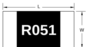
Fig. 5 Chip resistor outlines
