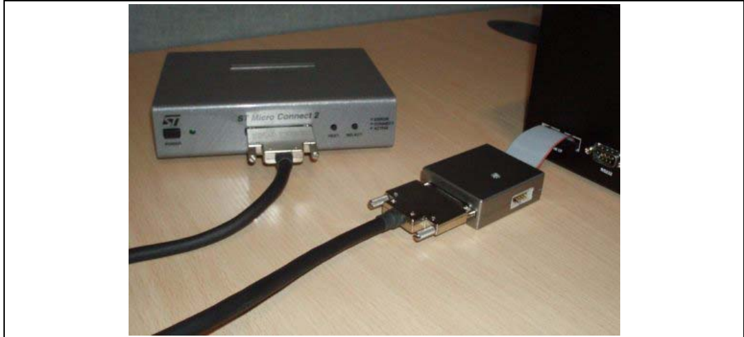
Figure 16. Connecting the STMC I/O convertor to an ST board
