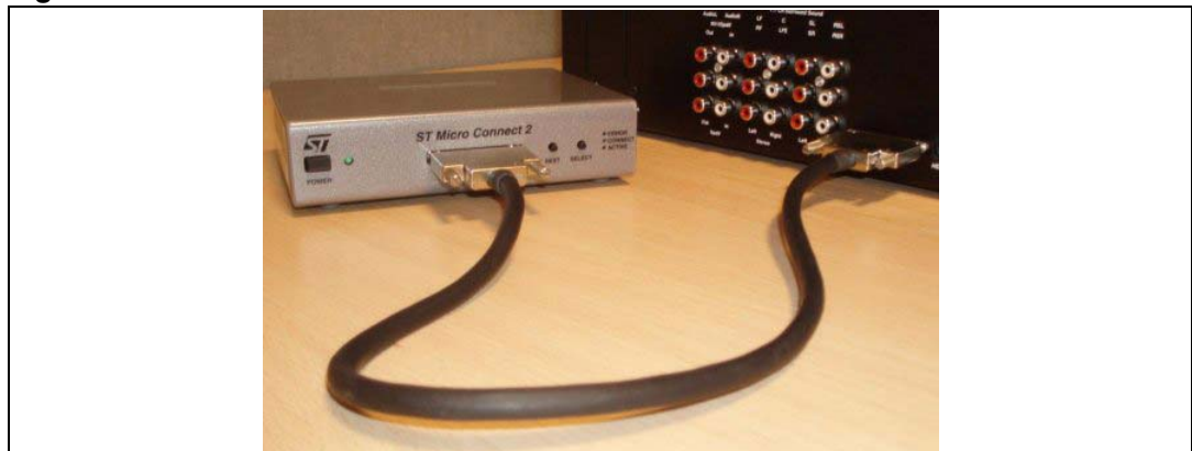
Figure 13. Direct connection to the ST Micro Connect 2
