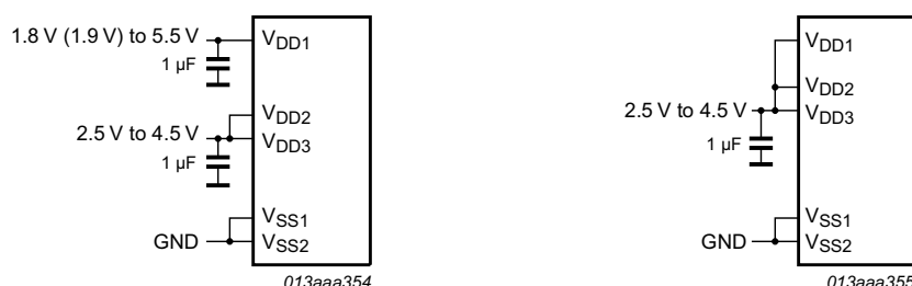
Fig 30. Recommended V_{DD} connections for internal V_{I,CD} generation
