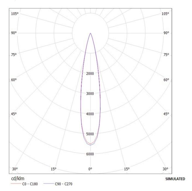
Luminaire: Ledil Oy FA10613\_LM1-RS FA10613\_LM1-RS Lamps: 1 x Cree MC-E (White)
