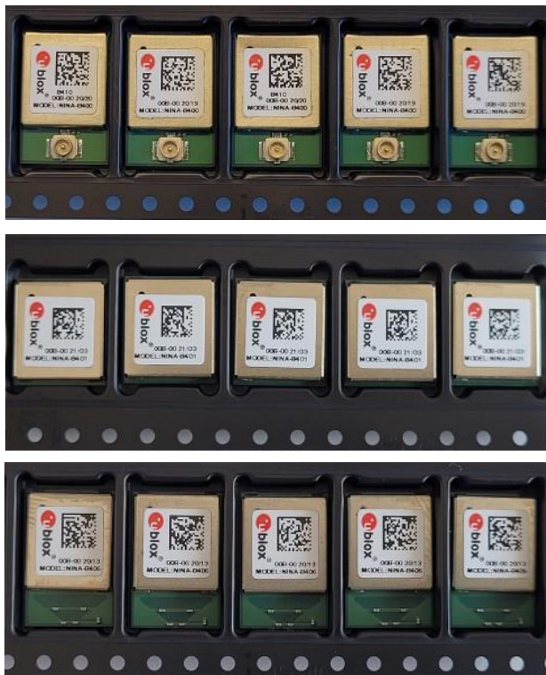
Figure 9: Orientation of NINA-B410/B411/B416 modules on tape
