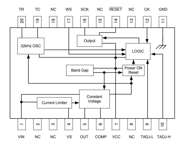
Note: Some of the functional blocks, circuits, or constants in the block diagram are omitted or simplified to clarify the descriptions of the relevant features.
