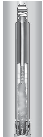
Vapor quenches arc at first current zero
