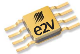
Figure 2. Package Type 8-lead CFP
