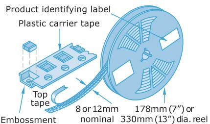
Tape and reel packing of surface mounting chip capacitors for automatic placement are in accordance with IEC60286-3.
