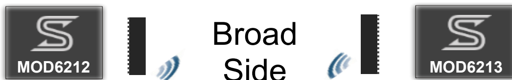
Figure 8.2. Broad Side Antenna Configuration
