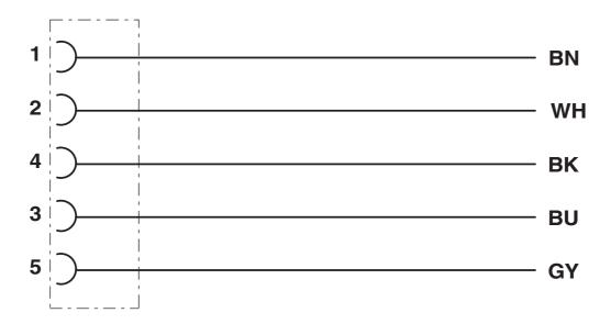
Contact assignment of the M12 socket
